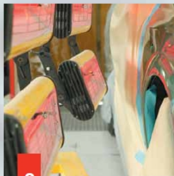
8 Infrared drying topcoat
