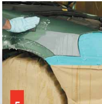
5 Panel preparation with Blend-Prep
